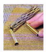
Step Two: Rough up the pen tubes so the glue will have a good bonding surface with the tube and the inside of the cactus.
