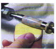
Step Seventeen: Use the PFK-1 cushioned abrasive pads to wet sand the ca finish.
