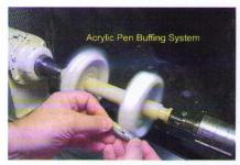
Step Eighteen: Use the specially designed Acrylic Pen Buffing System
